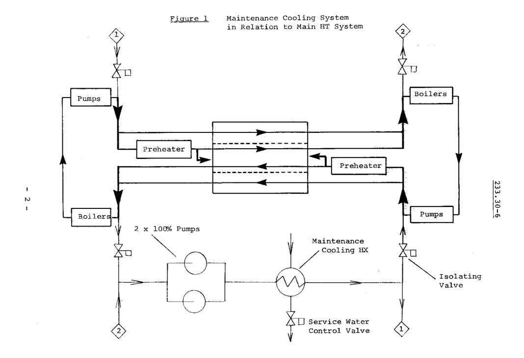
During normal operation, the system is isolated from the main HT system, and is filled with nitrogen gas to minimize corrosion. Prior to use, the system is filled with HT  $\rm D_2O$ , usually from central storage. Adequate venting of the system must be provided, typically to the HT  $\rm D_2O$  collection system whose leakoff flow guages will indicate when the system is full.
